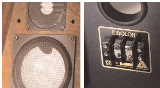
Grille-off shots reveal ceramic mid and treble drivers; underside view connecting terminals and bass vent
